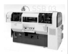
The SSB-02 2 cavity stretch blow moulding machine produces 2800 bottles/hour of 0.2L to 5L capacity whereas SSB-03 3 cavity stretch blow moulding machine produces up to 3600 bottles/hour of 0.2L to 1L capacity.
